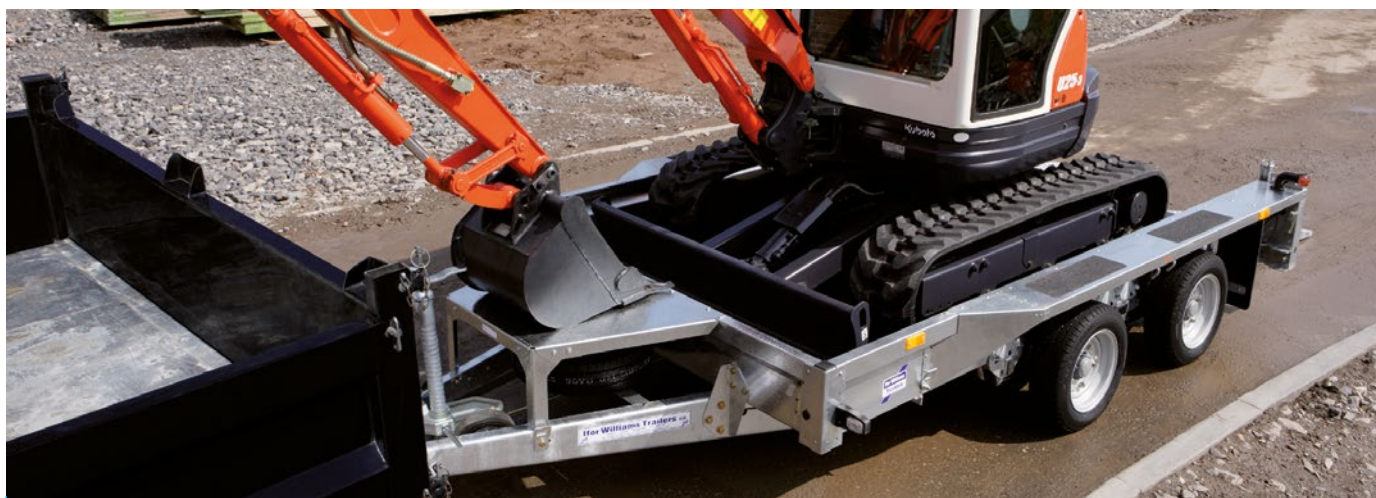
GX106 with skids and integrated rear supports
