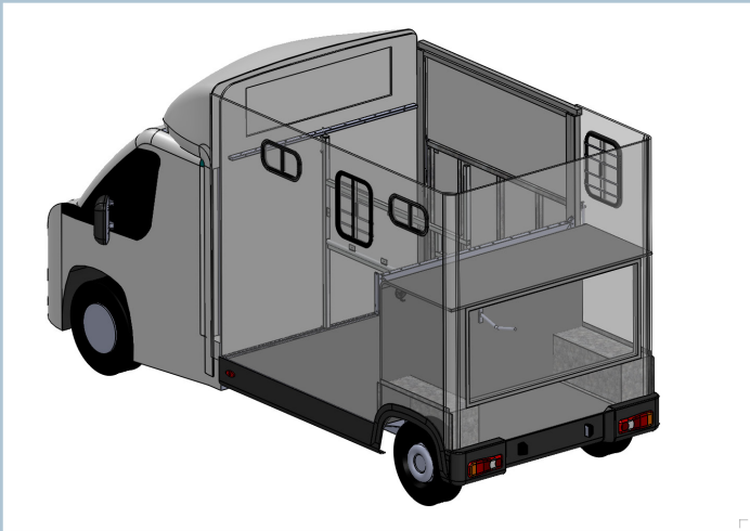
Option 3 (Rear Tack Locker): Single large tack/grooms locker accessed via external lockable door to the rear
