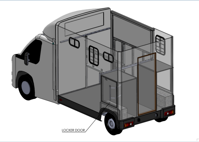
Option 2 (External Tack Lockers): Dual enclosed tack/grooms lockers accessed via external lockable doors
