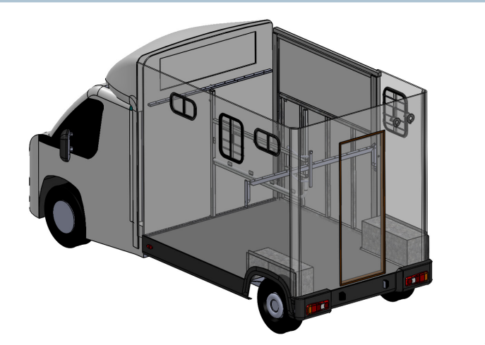
Standard Model Layout: No Tack Lockers
