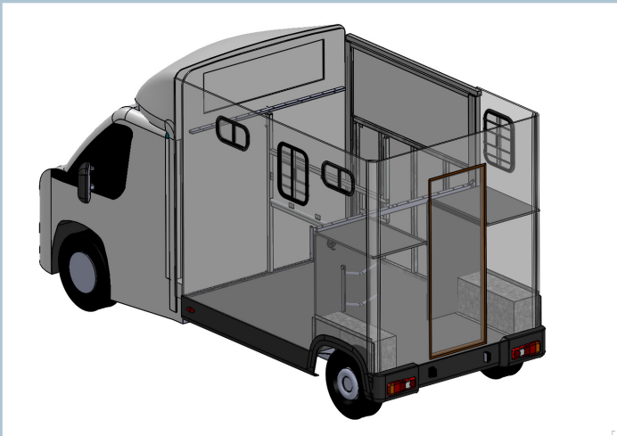
Option 1 (Internal Tack Lockers): Dual open tack/grooms lockers accessed from within the horse area
