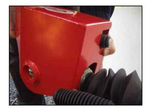
**2.** Tilt the rear of the red hitchlock cover back and "feed" the handle through the slot provided.
