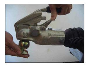
**1.** Lift the handle and insert the dummy ball ensuring the handle returns to the fully down position.
