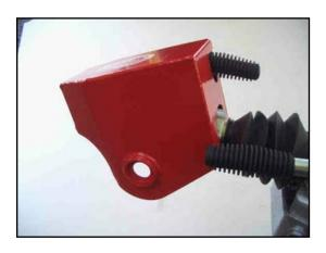
**3.** Pivot the red cover down towards the front so it rests on top of the hitch.
