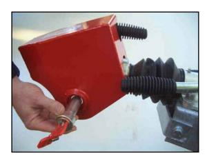
**4.** With the lock bar in the unlocked position, insert it into the red cover and push it into the lock housing. When in position, turn the key ½ turn clockwise to lock and remove key.
