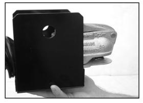
2. Offer up bottom channel according to your hitch type. Short fill strip at front for 12 - 14304 or tall fill in strip at front for 12 - 15851.
