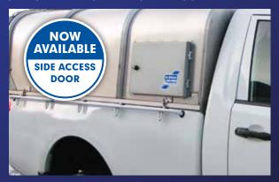
A versatile side access door is available for most pick-up and trailer canopies. The door can be fitted to the drivers' side or passenger's side between any of the roof channels.
