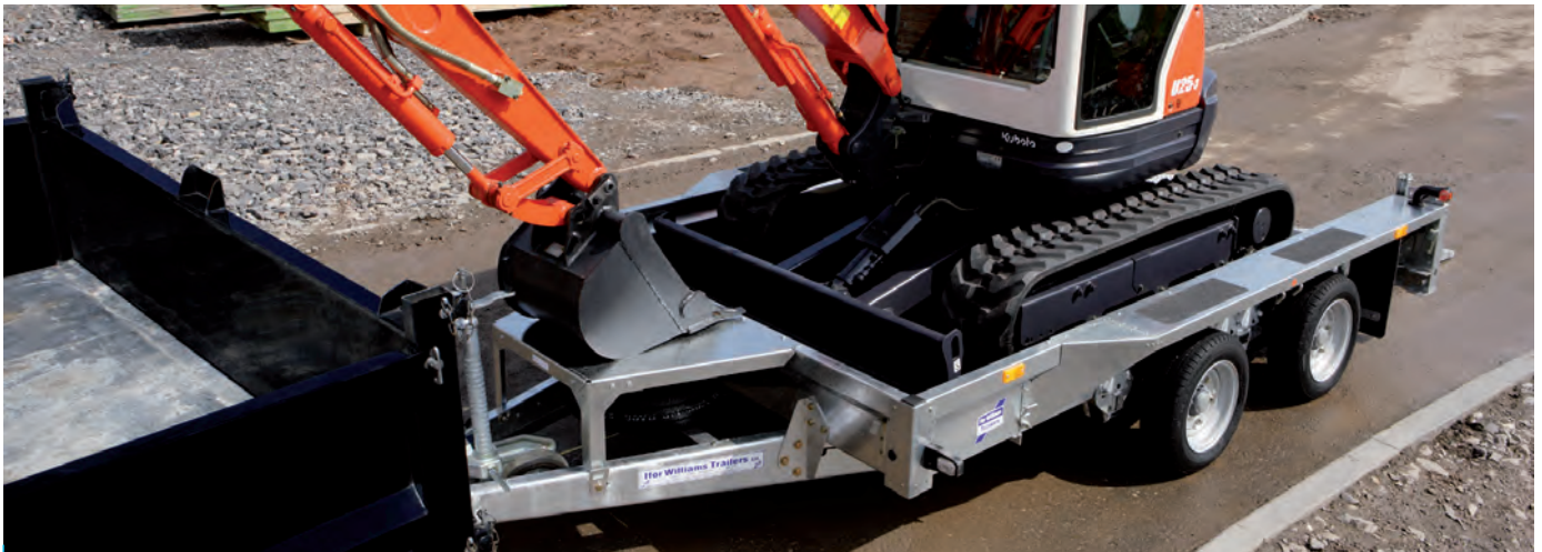
GX106 with skids and integrated rear supports
